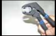
Open the plier and slide the clamp over the sheet metal edges to be joined and release the pliers
